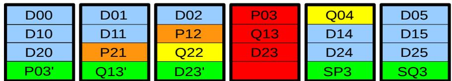
Figure 7: Degraded VDEV with Distributed Hot Space
