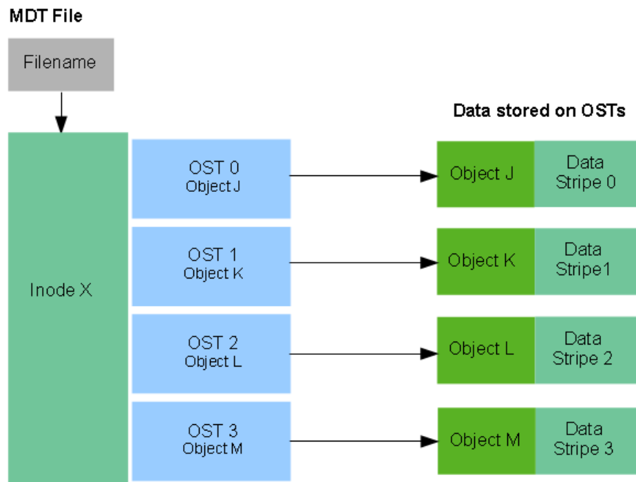
FIGURE 1-3 MDT file points to objects on OSTs containing file data
